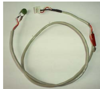
Figure 1. The temperature sensor, based on a 10 Ohm NTC thermistor and a precision resistor. Note that the resistor is near the controller input, and the thermistor is farther away (30 cm of cable) to minimize common mode errors due to the heating of both components.
