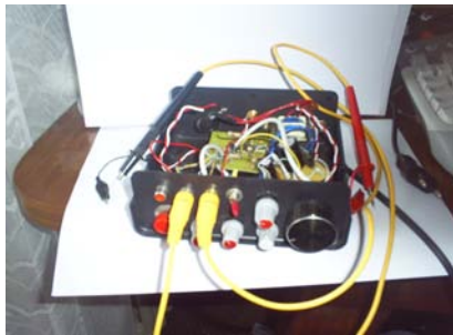
Figure 3. The signal generator used in testing the neural network, built around an EXAR 8038 precision waveform generator chip and momentarily powered from an external filtered tracking supply (not shown).
